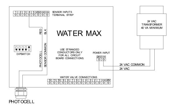
TRANSFORMER NOTE: Use machine tool variety, 40 VA minimum is recommended. If a larger transformer is used, adjust the fuse protection accordingly.
