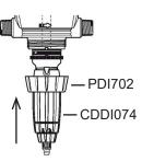
18. Cut 1" off from the top of the suction hose to ensure a tight fit, make sure to cut in
