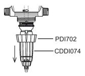
5. Unscrew the locking nut (PDI733) from the injection stem assembly (CDDI074) and remove the black anti-rotation
