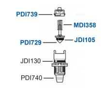
14. Insert the new check valve assembly (PJDI115) back into the bottom of the injection stem assembly (CDDI074) and screw the check valve nut (PDI734) back on.
