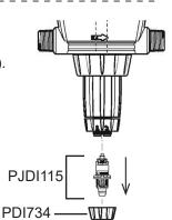
3. Take off the top guide (PDI739) by giving it a 1/4 turn counter clockwise, and discard. Discard the check valve spring (MDI358), check valve cone (PDI729) and check valve cone o-ring (JDI105).
